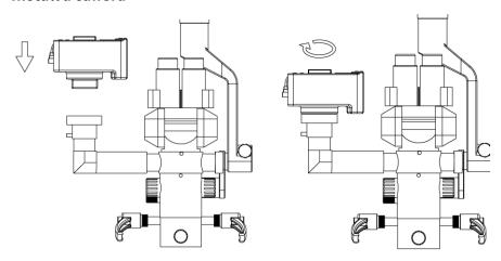
把相机装到分光镜筒上(相机装到相机卡口时,要对准卡位,然后旋转相机,直到听到"咔"的一声表示相机装好了) Install a camera to the light splitter tube (Aim at snap points when the camera install to a snap joint and then rotate a camera untill hear a sound of "ka" a camera installation is ok
